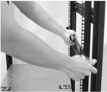
1. Secure the side rails to the rack.
