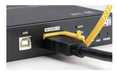
3 Wrap the tail tightly around the HDMI cable.
