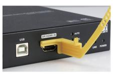
2 Connect the HDMI cable to the HDMI section (lower side) of the DisplayPort/HDMI combo connector.
